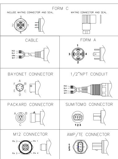
$\label{Note:Refer} \textbf{Note:} \ \ \textbf{Refer to installation instructions supplied with devices for recommended torque.}$
